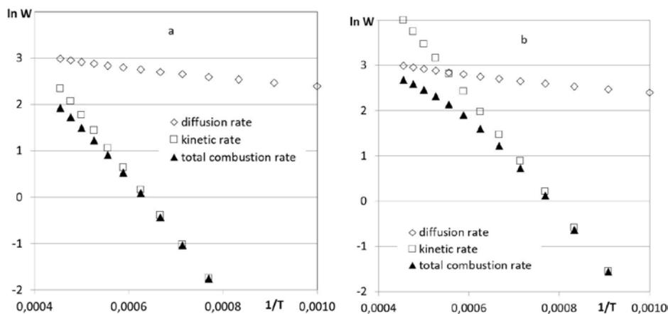
Fig. 4. Dependence of the logarithm of the specific combustion rate  $W$ , c-1, on the temperature, K-1, for pulverized particles ( $d = 50 \mu m$ ) of coke residue: a – of anthracite, b – of bituminous coal
