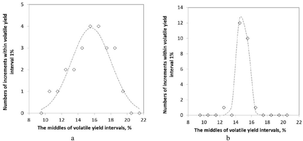
**Fig. 1.** The example of  $V^{daf}$  values distribution in increments of the lot of mixture of anthracite with bituminous coal, prepared at the TPP coal storage place: a – sampled from coal pile, mean value  $V^{daf} = 15.5\%$ ,  $SD = 2.4\%$ ; b – sampled from raw coal bin feeder, mean value  $V^{daf} = 14.9\%$ ,  $SD = 0.6\%$
