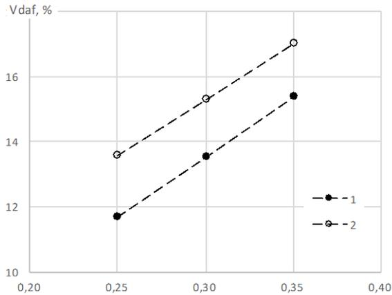
**Fig. 2.** The dependence of volatile yield of the mixture on the share of bituminous coal, with volatile yield of anthracite: 1 -  $V^{daf} = 5.0\%$ , 2 -  $V^{daf} = 2.5\%$
